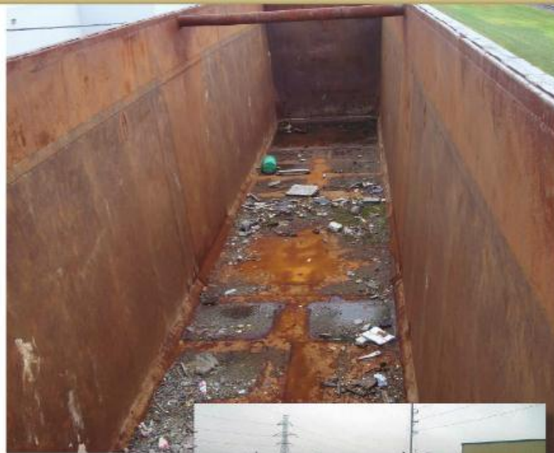
TOP: 5,700 cubic cube car for C&D transport. RIGHT: 89' 70 ton flat at transfer station.
