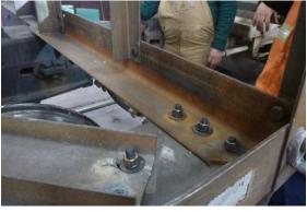
In the picture to the left, you can see where the repairs that were made whereby the repairing party replaced part of the end sill with steel angle instead of aluminum. If you're not familiar, aluminum and steel are not incompatible metals. Anytime two dissimilar metals come into contact, you run the risk of creating a corrosive environment whereby one of the
